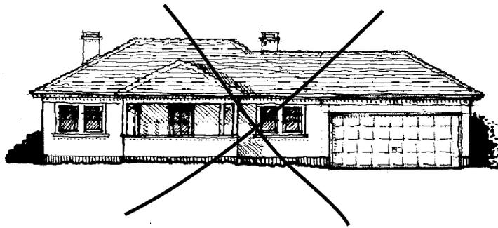
**Incorporating a garage under the roof line alters the form and scale of the dwelling**
